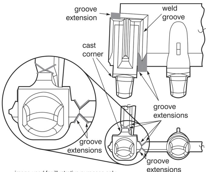
Groove Extensions, commonly referred to as "starter tabs" or "run-off tabs", are used to keep the starts and stops of the weld passes out of the final weldment. Tabs should be constructed of 1/4" (6mm) thick mild steel (ASTM A36 or equivalent) and extend at least 2" (50mm) beyond the ends of the weld grooves. Tabs will be removed by the air carbon arc gouging process at the completion of the weldment.
