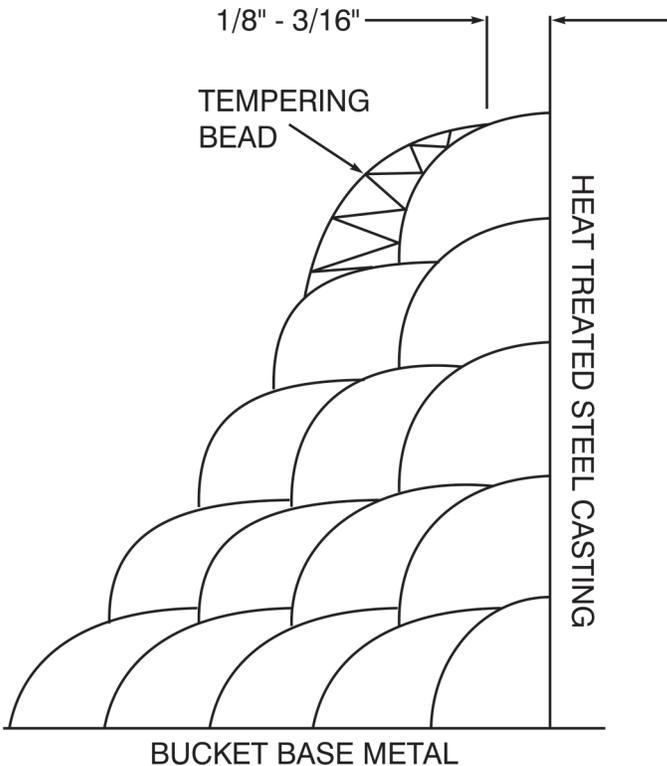
Tempering or annealing weld pass is used in all weld joints that weld is deposited against the heat-treated steel castings. It is an additional weld pass that is added to the weldment once the weld joint is completely filled.
