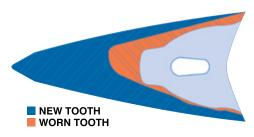
The XS RC style tooth shown here offers a consumption ratio of 60%.
