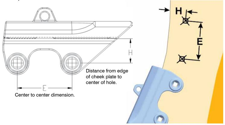
Once the dimensions have been confirmed, at each center mark drill a 1-1/16" diameter hole using a magnetic drill. Install the proper plow bolt assembly (refer back to shroud dimensions table for this assembly). A cone nut is required for this installation. Torque to 500 ft-lb minimum and 600 ft-lb maximum.
