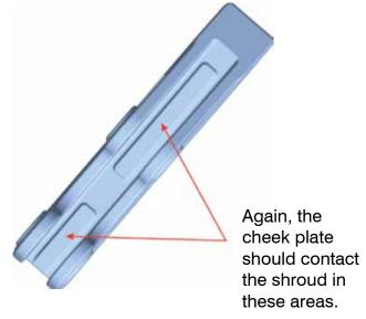
Once the shroud is on the cheek plate and has bottomed out, move the shroud towards the lower shroud until a gap of 1/4" - 1/2" is reached. This gap must be maintained during the rest of the installation.
