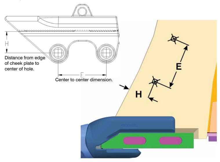
Once the dimensions have been confirmed, at each center mark drill a 1-1/16" diameter hole using a magnetic drill. Install the proper plow bolt assembly (refer back to shroud dimensions table for this assembly). A cone nut is required for this installation. Torque to 500 ft-lb minimum and 600 ft-lb maximum.
